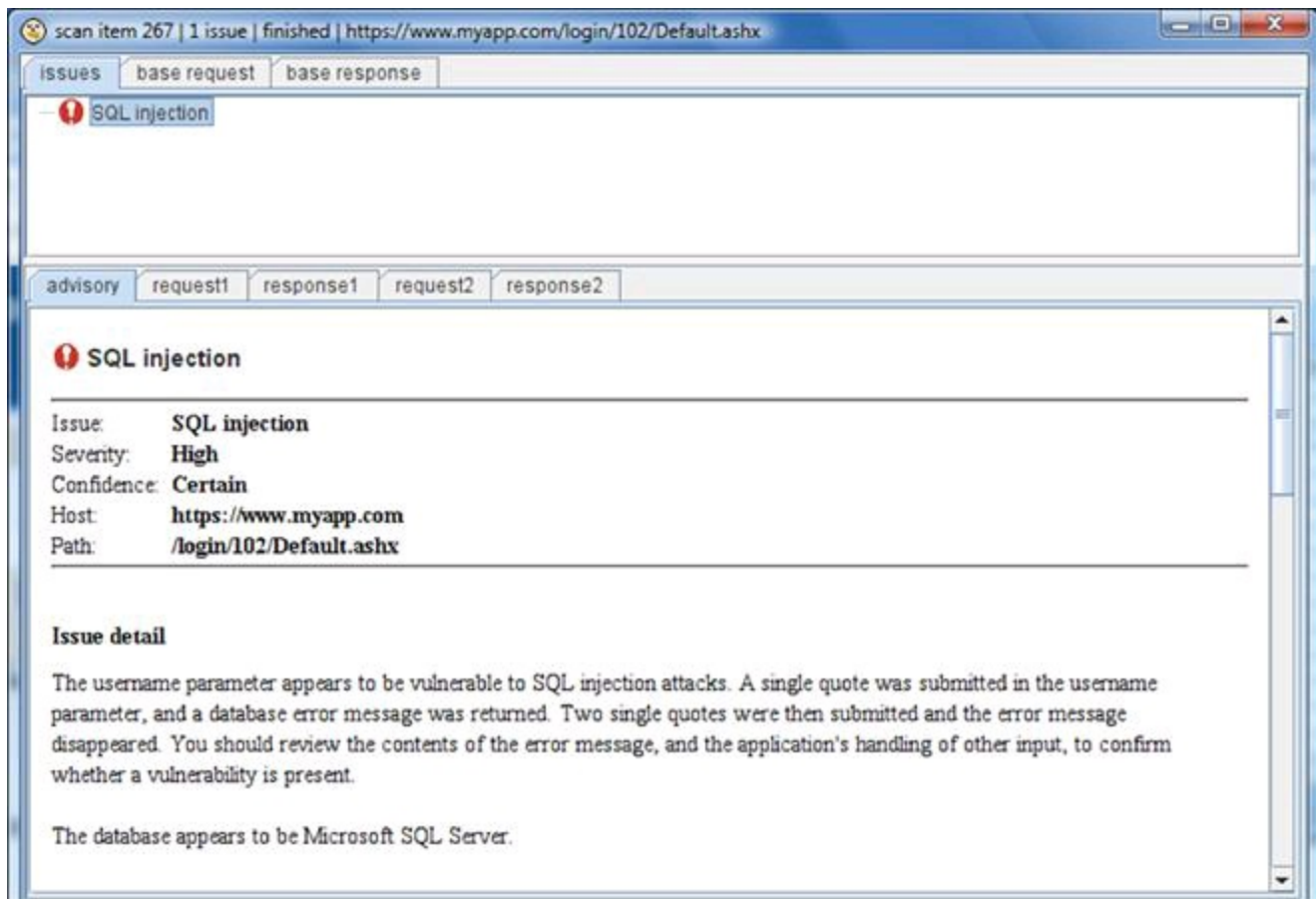
FIGURE 3.20 Single item review in Burp Scanner.
